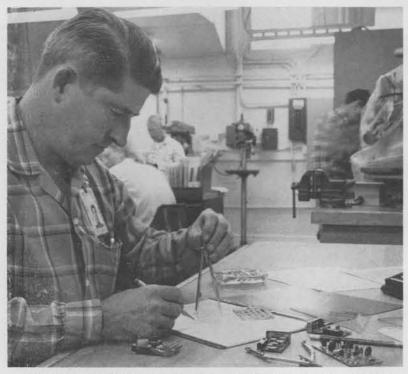
LAYOUT of printed circuit and visualization of the finished component is performed by Bob Higley from design engineer's schematic drawing and packaging requirements. Bob's work then goes to a draftsman for final drawing of the circuit to be printed.
